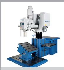
Floor Plate (Pos. 2.10) with swivable cube (Pos. 2.80) at the reverse side, with swivable table (Pos. 2.40) aside
